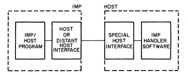
The Host (or Distant Host) Interface and the Special Host Interface communicate according to the hardware specification set down in BBN Report No. 1822, *Specifications for the Interconnection of a Host and an IMP*, and the IMP/Host program (in the IMP) and the IMP Handler software (in the Host) communicate using the software protocol described in the same document.
